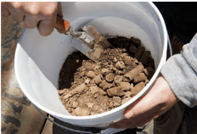
Figure 6. Use a clean hand tool to mix the subsamples
